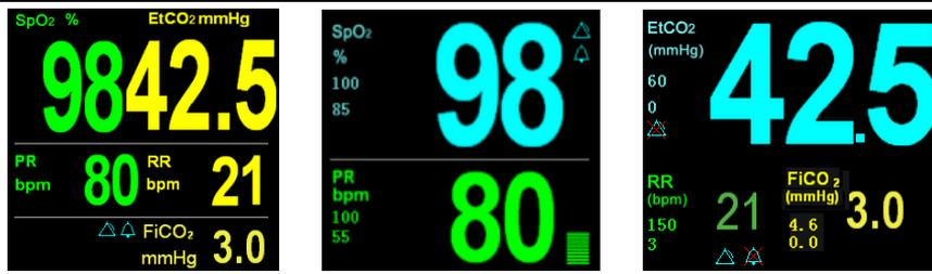
(a) SpO<sub>2</sub> and CO<sub>2</sub> Module (b) SpO<sub>2</sub> Only (c) CO<sub>2</sub> Only
