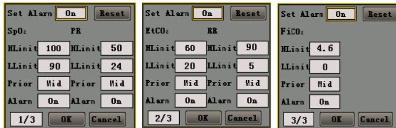
Figure 5-7: SpO<sub>2</sub> and CO<sub>2</sub> Set Alarm limits
